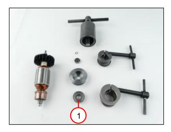
1. Pull ball bearing (1) off armature.
