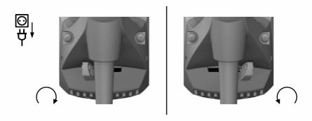
• Set the forward / reverse selector switch to forward or reverse rotation.
